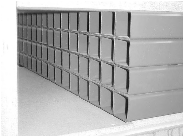
Fig. 9.20. Photograph of a duct wall lined with resonators which are realized by rigidly terminated pipes of depth d
